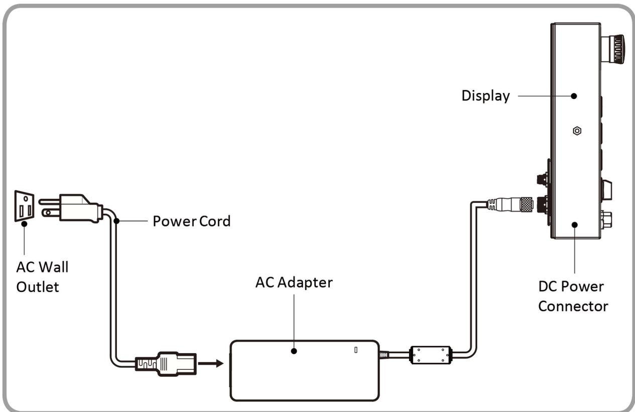
AC Adapter specifications and display power consumption vary by LCD panel size.
