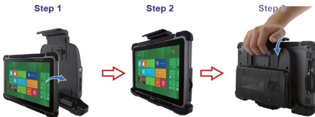
1. Lower the tablet with its top slightly tilted forward into the vehicle mount. Align the docking alignment fingers on the bottom of the vehicle mount to bottom of the tablet where the two alignment holes (to the sides of the pogo-pin) are, then push the tablet in against the vehicle mount.
