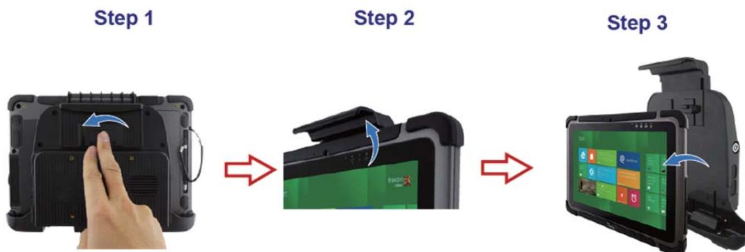
1. Reach for the latch on the back of the tablet and pull it sideways.
